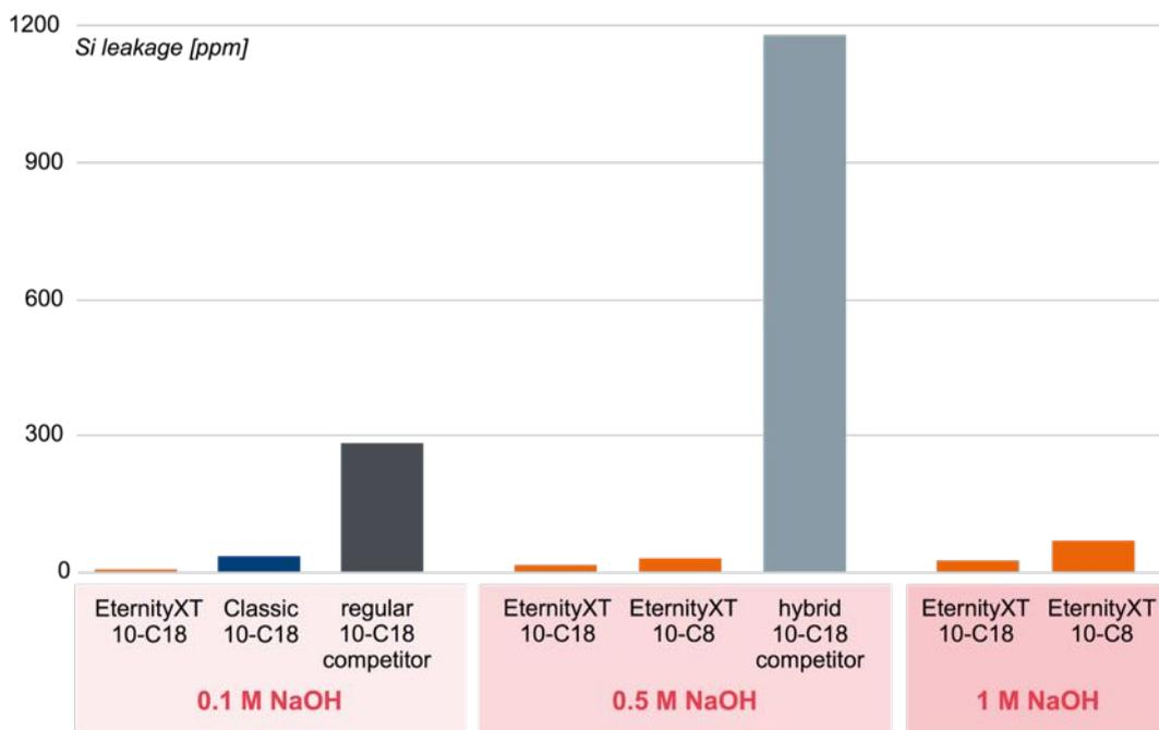
The figure shows the leakage of silicon during after a number of CIP cycles at different NaOH concentrations. At 0.1 M NaOH, even Kromasil Classic resists better than regular competitors. Already at 0.5 M NaOH, the main hybrid 10-C18 competitor shows serious leakage, actually higher than EternityXT phases at 1 M NaOH.
