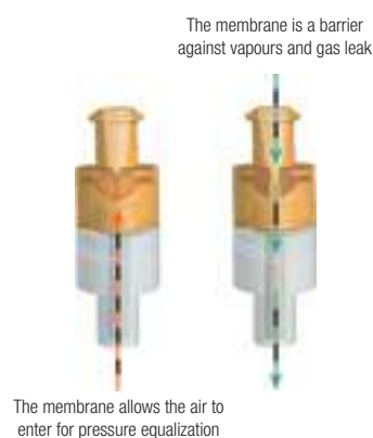
Figure 2. One-way check valve
