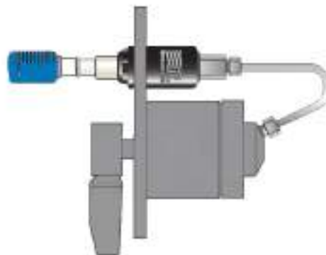
Figure 3. Suggested mounting arrangement of Model 7010 with filler port 7012
