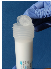
2 - Remove the PPHD Insert
