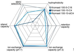
Kromasil<sup>®</sup> diC4 has strong C4 characteristics in terms of capacity and hydrophobicity. The main difference is a steric selectivity in between a C18 and a C4, more like a C8.
