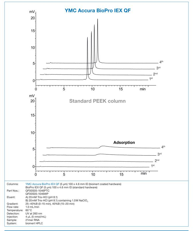
Oligonucleotides generally exhibit poor peak shape and therefore low recovery in AEX analysis, mainly due to adsorption onto the column hardware. YMC Accura BioPro IEX columns provide high recovery and very good peak shapes from the first injection. This makes YMC Accura BioPro IEX QF columns ideal for the analysis of oligonucleotides with reproducible results. The columns show stable peak areas from the 1<sup>st</sup> injection, so that no preconditioning is required.
