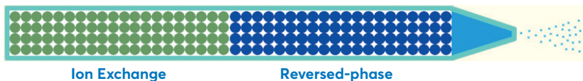
Figure 49. Multidimensional Protein Identification Technology (MudPIT) consists of an initial fractionation of a protease digestion of an entire proteome by ion exchange chromatography followed by a lengthy reversed-phase separation of the peptides from each fraction of the ion exchange separation. Narrow capillaries are packed with ion exchange beads and reversed-phase beads and the eluent from the chromatography is directed into an electrospray mass spectrometer.
