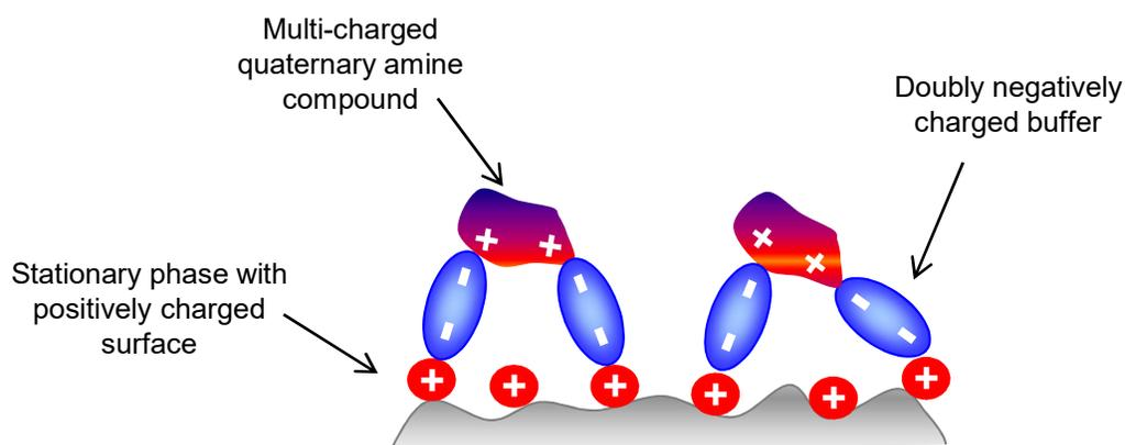
**Figure 5. Interaction of multi-charged quaternary amine with positively charged stationary phase**
